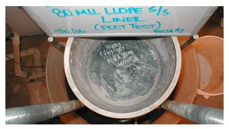
Figure 5 – 2.0 mm LLDPE, post-test.
