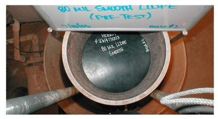
Figure 2 – 2.0 mm LLDPE geomembrane, pre-test.
