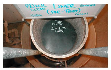
Figure 2 – 2.0 mm LLDPE geomembrane, pre-test.
