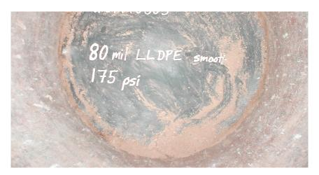
Figure 3 – 2.0 mm LLDPE, post-test.
