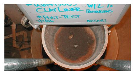
Figure 6 – Clay liner, post-test.
