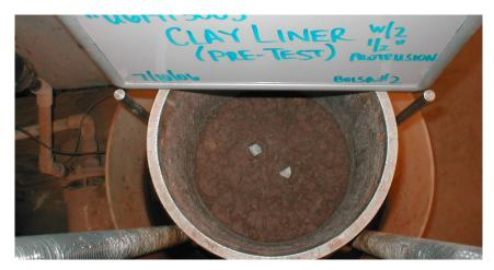
Figure 1 – Clay liner with rock protrusions, pre-test.
